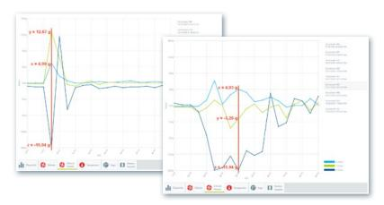
The course of a shock can be traced in milliseconds and per axis. As shown here in detail, the amount of acceleration per axis is not the only relevant factor, but also the duration of the shock. This allows serious damage to be detected.
